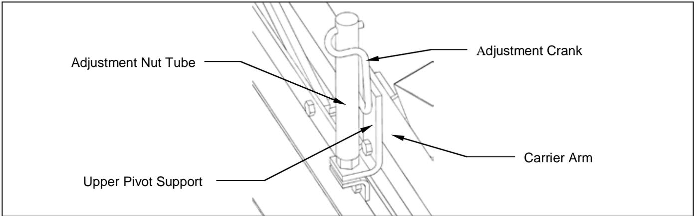
Figure 8: Securing Crank While Not In Use
